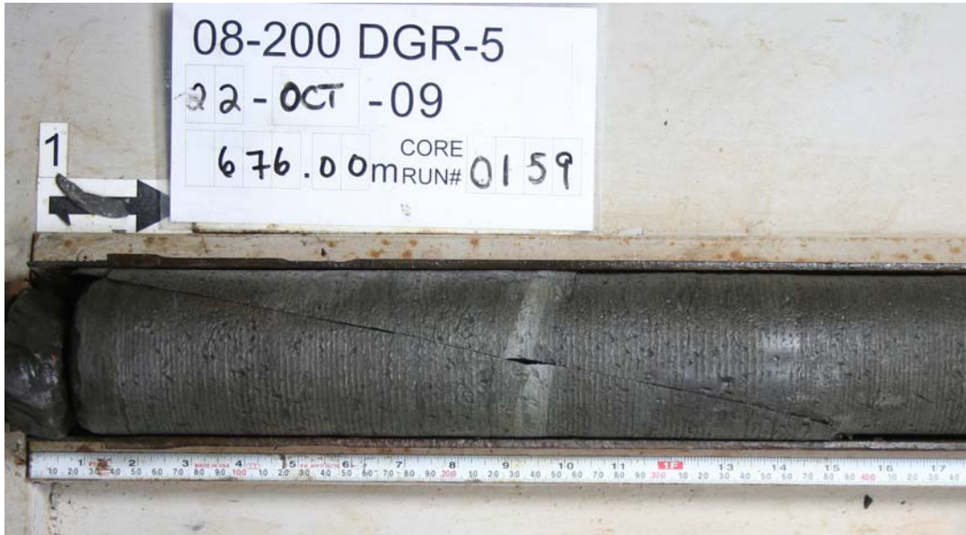
Figure 6 Inclined Fracture in DGR-5 at 676.18 mLBGS (MS Unit 3, Blue Mountain Formation). Note the Apparent Offset Along the Fracture is Not True and is Due to Misalignment of the Core Pieces
