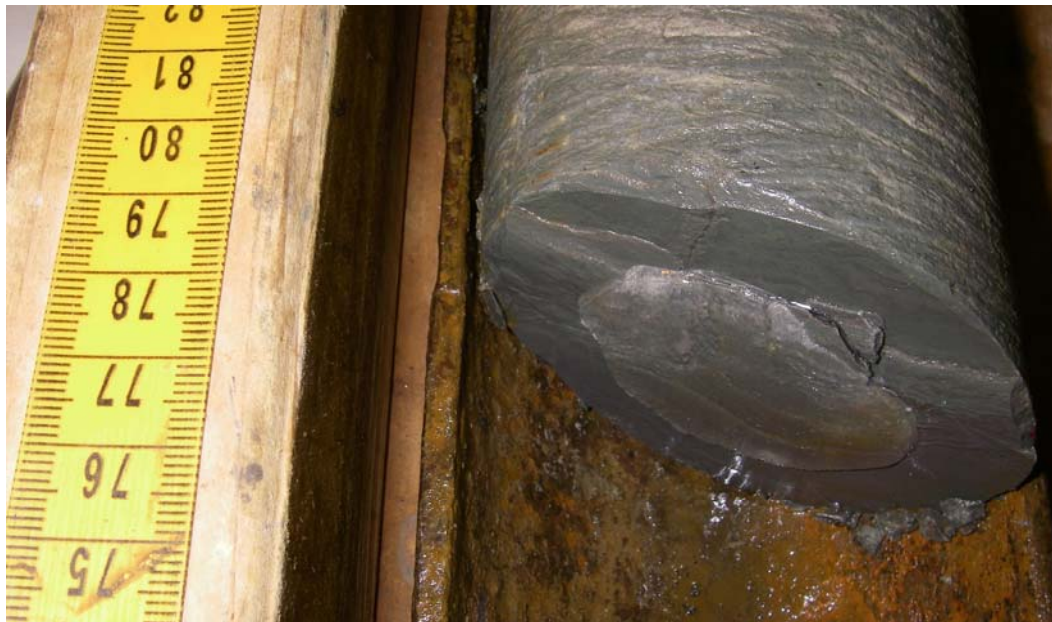
Figure 5 Bedding Fracture in DGR-6 at 504.93 mLBSG with Halite Infilling (MS Unit 3, Manitoulin Formation)
